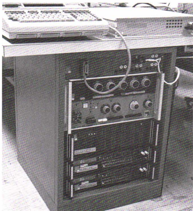
GPIB-based ATE allows rapid calibration of Racal-Dana products
