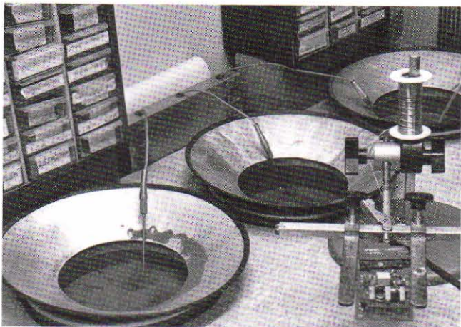
A proprietary zener-reference facility provides high quality references for Racal-Dana digital multimeters.
